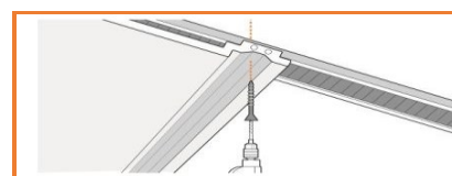
3.6 Shoot screws at prepared grooves. Shoot screws at every frame with a distance of no more than 40 centimeters.
